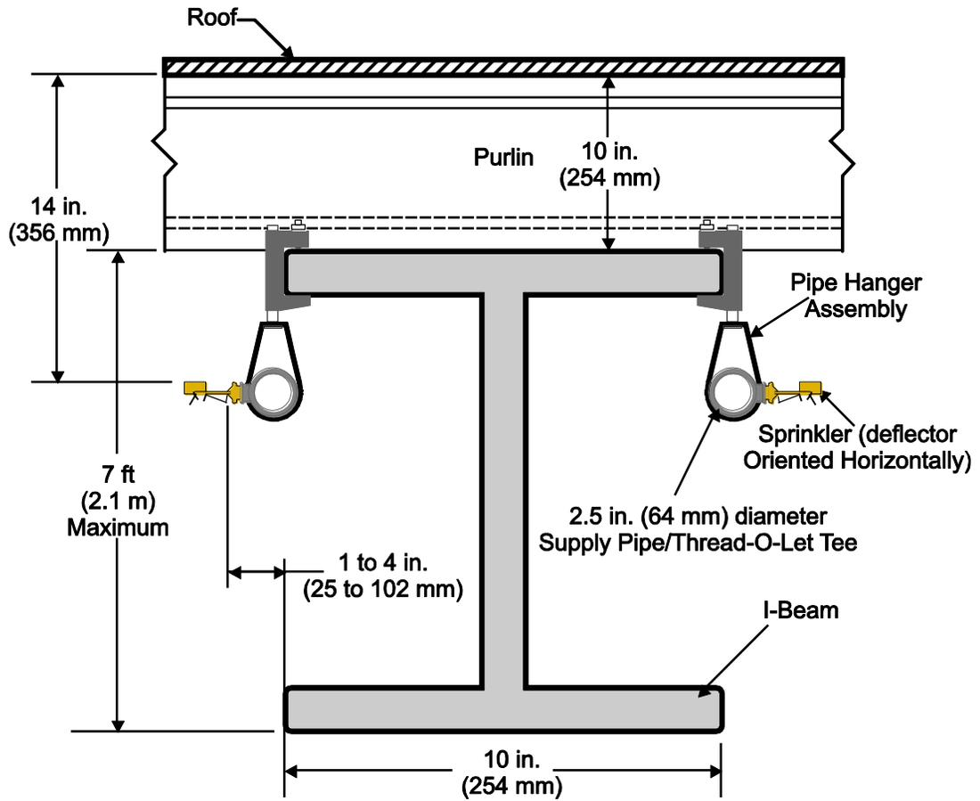
D-29: Sprinkler Installation Position K14.0 (K200) Non-Storage Extended Coverage Horizontal Sidewall Sprinkler
