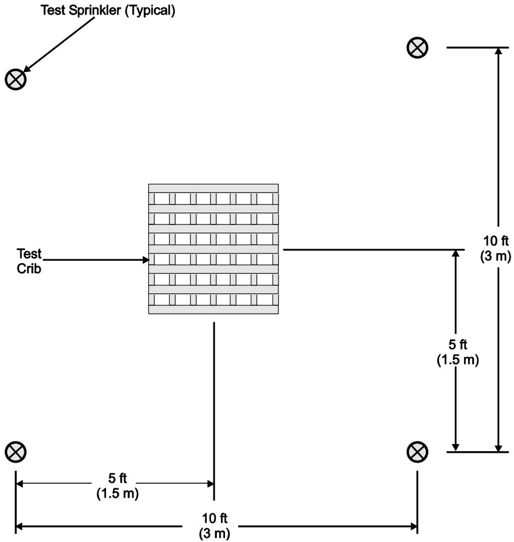
D-22: Crib Fire Test - Sprinkler Position with Respect to Crib
