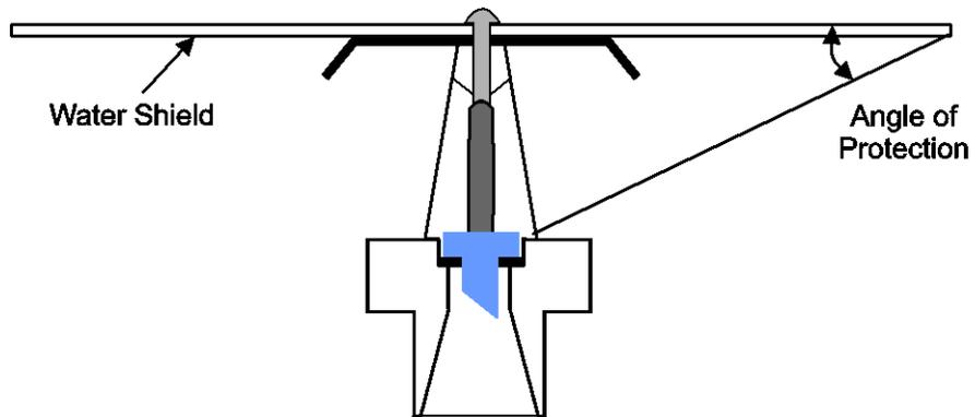
D-1: Impingement (Angle of Protection) – In-Rack Sprinkler
