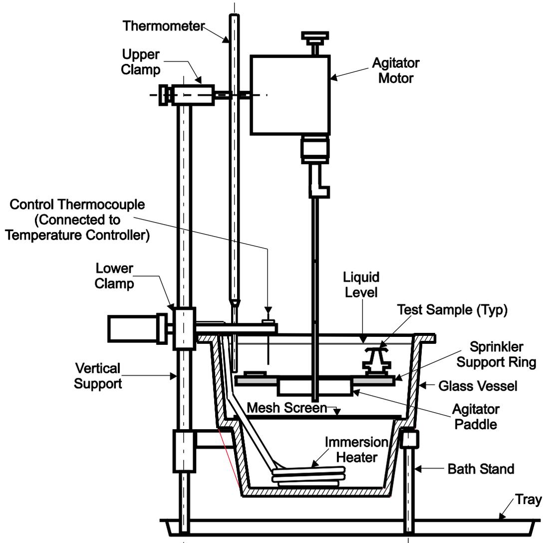
D-5: Operating Temperature (Liquid Bath) Typical Test Setup
