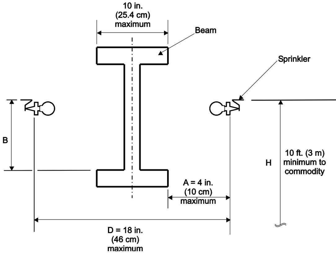
D-18: K14.0 (K200) Non-Storage Extended Coverage Horizontal Sidewall Sprinkler Location for Distribution
