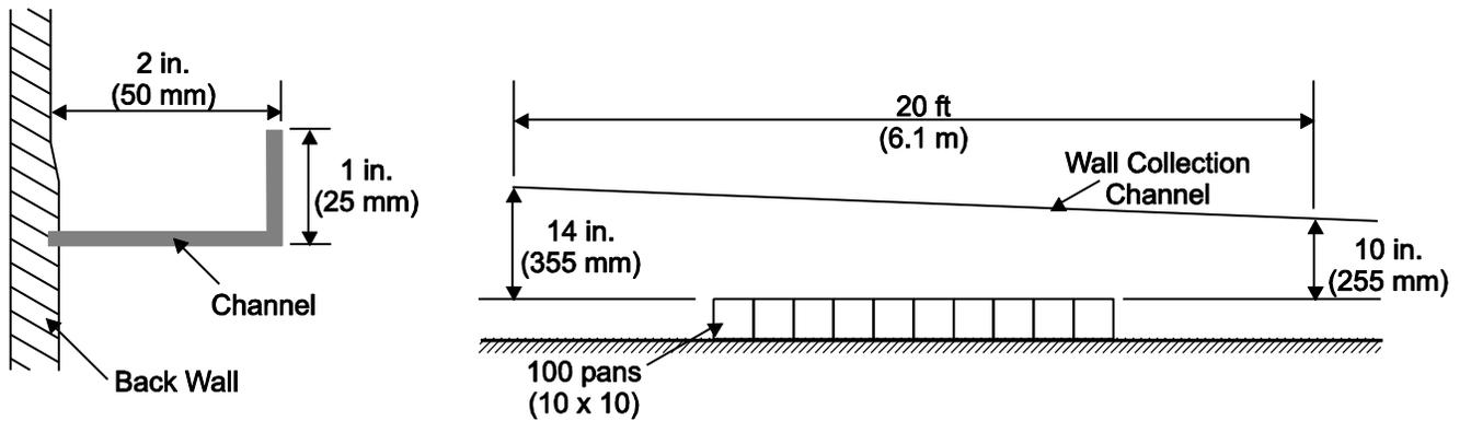
D-16: Standard Coverage Sprinkler Distribution – Test Setup for Sidewall Sprinklers (Detail)
