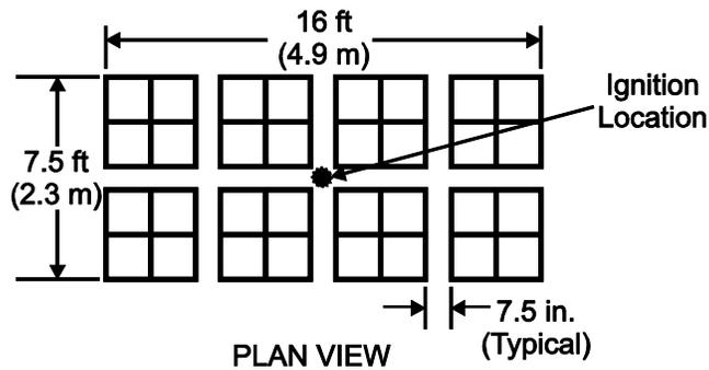
D-30: Full Scale Fire Test Array for K14.0 (K200) Non-Storage Extended Coverage Horizontal Sidewall Sprinkler
