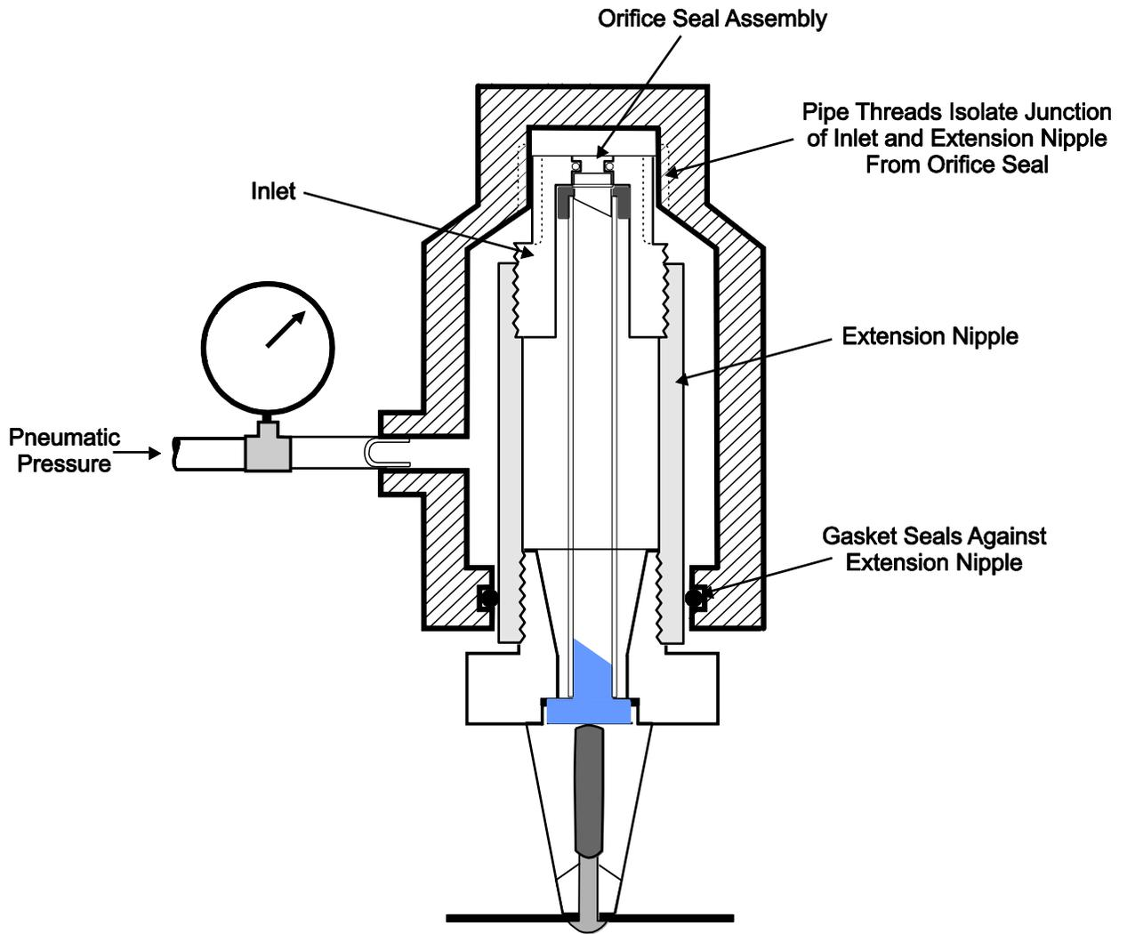
D-4: Pneumatic Leakage - Dry Sprinkler Inlet Test (Dry Sprinklers Only)
