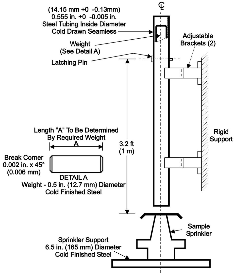
D-8: Rough use and Abuse (Drop Impact) Test Apparatus
