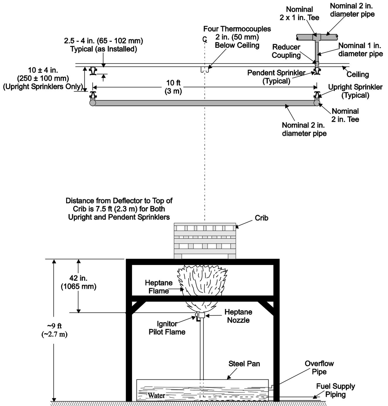
D-23: Crib Fire Test - Arrangement with Piping
