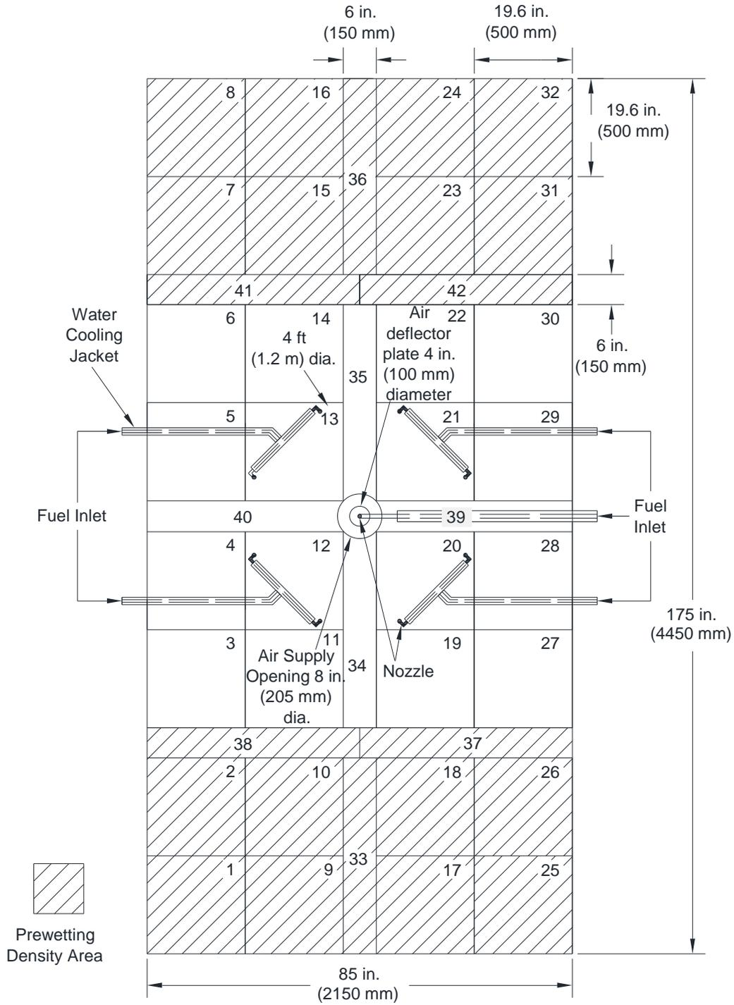
D-19: Actual Delivered Density (ADD) Apparatus – Plan View
