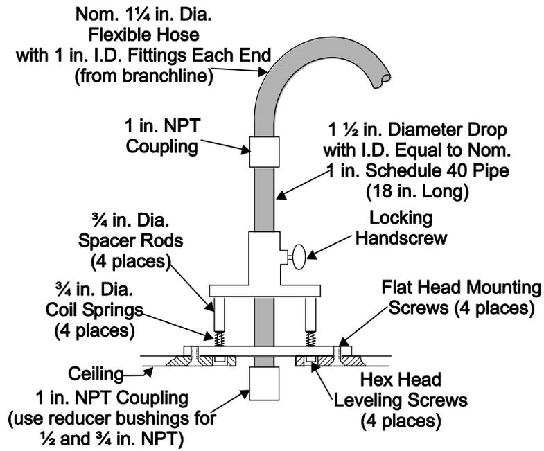
D-14: Standard Coverage Sprinkler Distribution - Adjustable Drop Detail for Pendent Sprinklers
