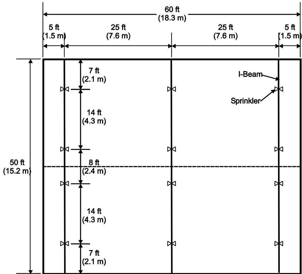
D-28: Sprinkler System Layout - K14.0 (K200) Non-Storage Extended Coverage Horizontal Sidewall Sprinkler
