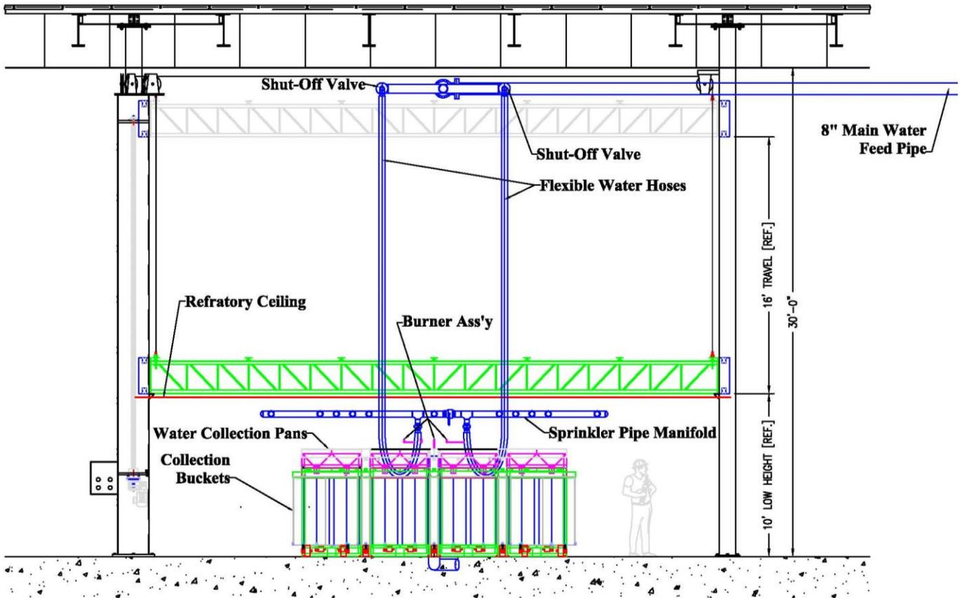
D-20: Actual Delivered Density (ADD) Apparatus – Elevation View
