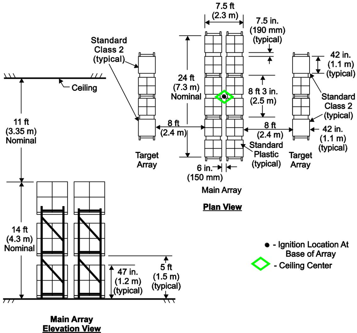
D-25: Full Scale Fire Test Array for K11.2 (K160) and K14.0 (K200) Upright and Pendent Storage, Test B
